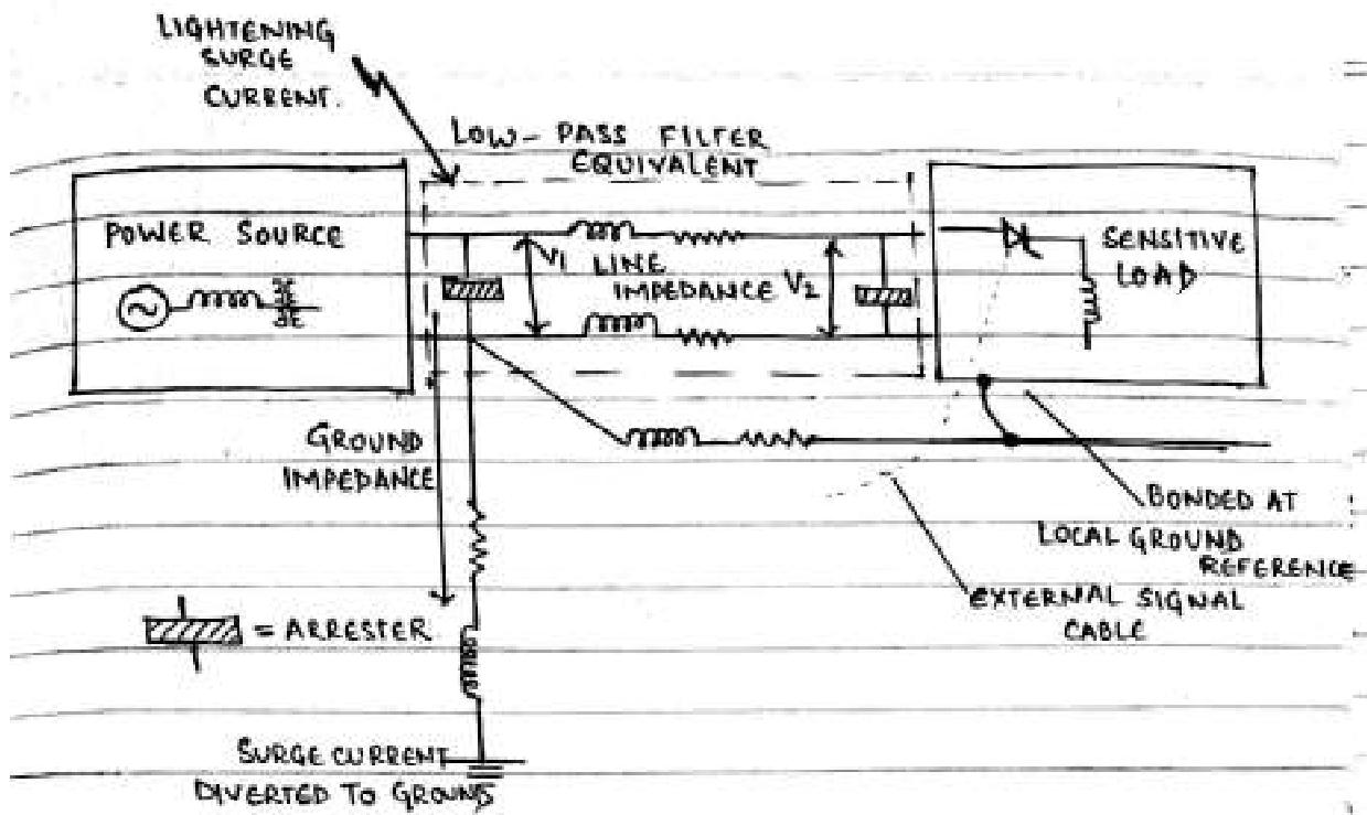
The first arrester is connected from the line to the neutral ground bond at the service entrance. It limits the line voltage  $V_1$  from rising too high relative to the neutral and ground voltage at the panel.
