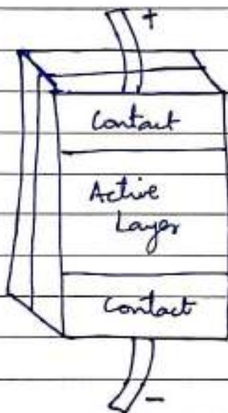
Fig. 8 Basic construction of LSA diode.
