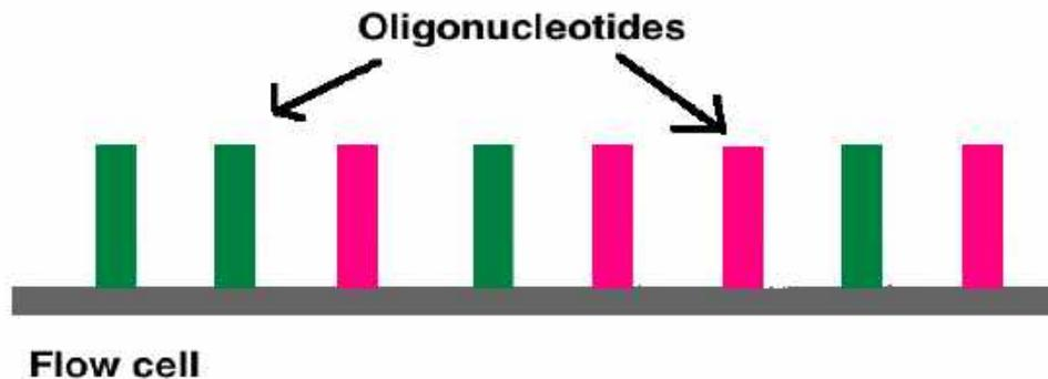
Millions of oligos line the bottom of each flow cell lane.
