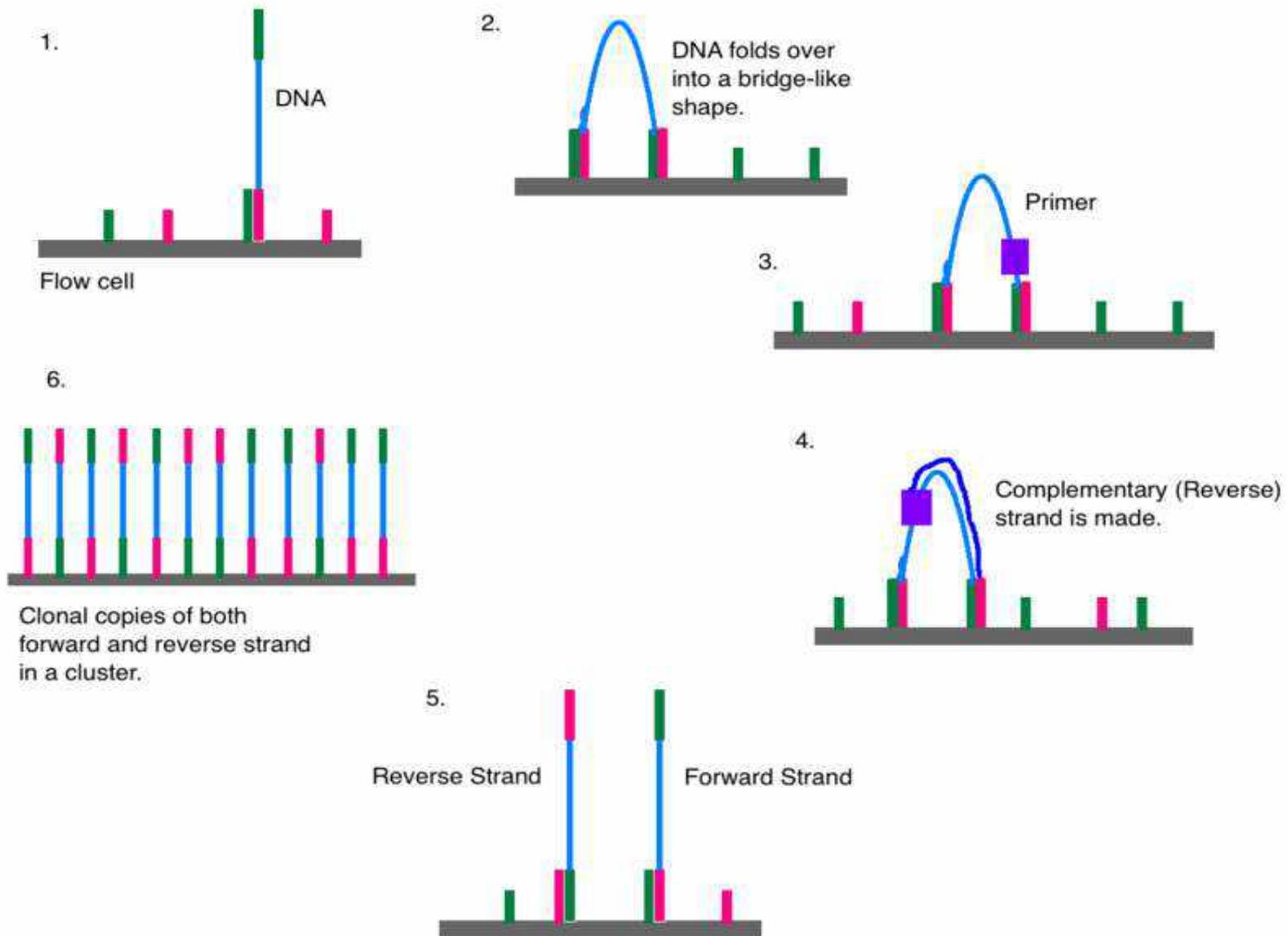
The DNA attaches to the flow cell via complementary sequences. The strand bends over and attaches to a second oligo forming a bridge. A polymerase synthesizes the reverse strand. The two strands release and straighten. Each forms a new bridge (bridge amplification). The result is a cluster of DNA forward and reverse strands clones.
