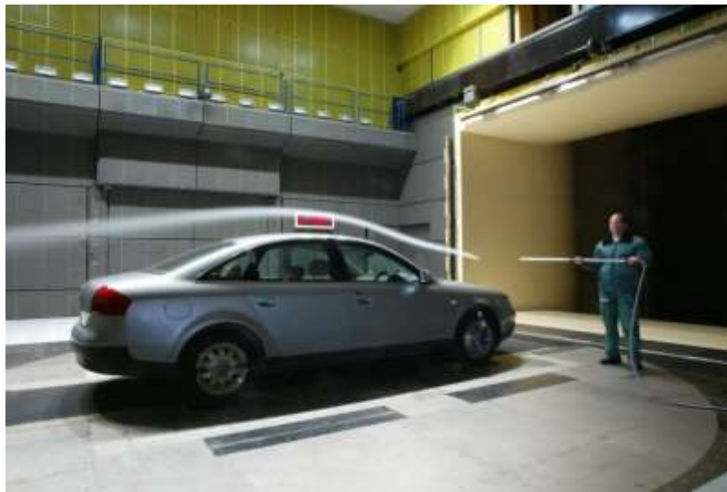
Example of a streakline used to visualize the flow around a car inside a wind tunnel.
