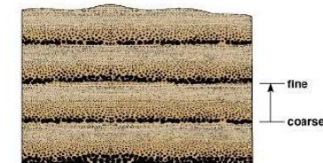
The figure above shows normal grading , where grain size gets smaller moving up section.
